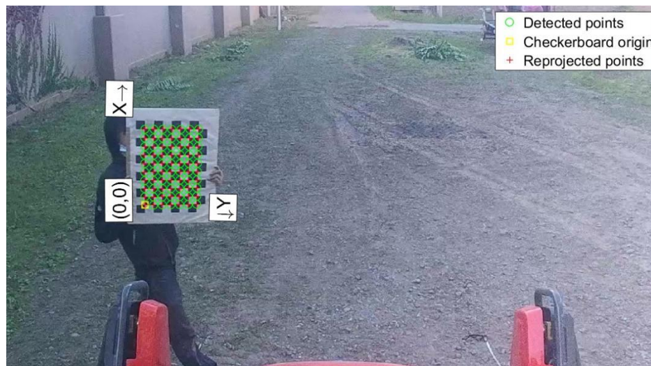
Figure 4.2-2 Multiple shots of a chessboard grid at different positions for camera calibration.
