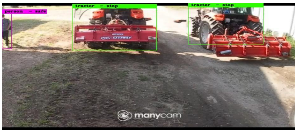
Figure 3.5-1 The remote safety system detection results.
