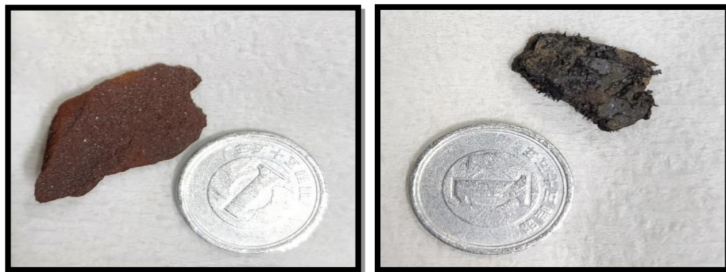
Figure 3.8 High-Purity iron oxide specimens used as working electrode; hematite (left) and magnetite (right), respectively.
