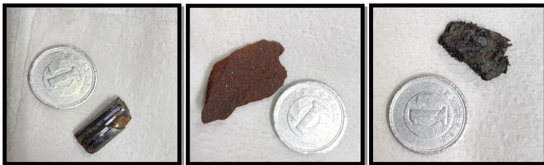
Figure 4.1 Ore specimen used as improvised working electrode a) Rutile, \text{TiO}_2 b) Hematite, \text{Fe}_2\text{O}_3 and c.) Magnetite, \text{Fe}_3\text{O}_4 .
