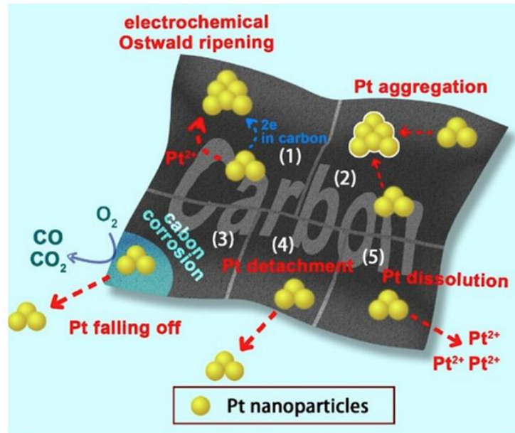
Figure 1-6. Schematic diagram of the performance loss mechanism of Pt/C catalysts in ORR.
