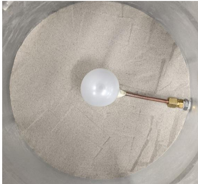
Figure 5.3. Soil with cavity preparation and Balloon insertion within soils layer at desired position.
