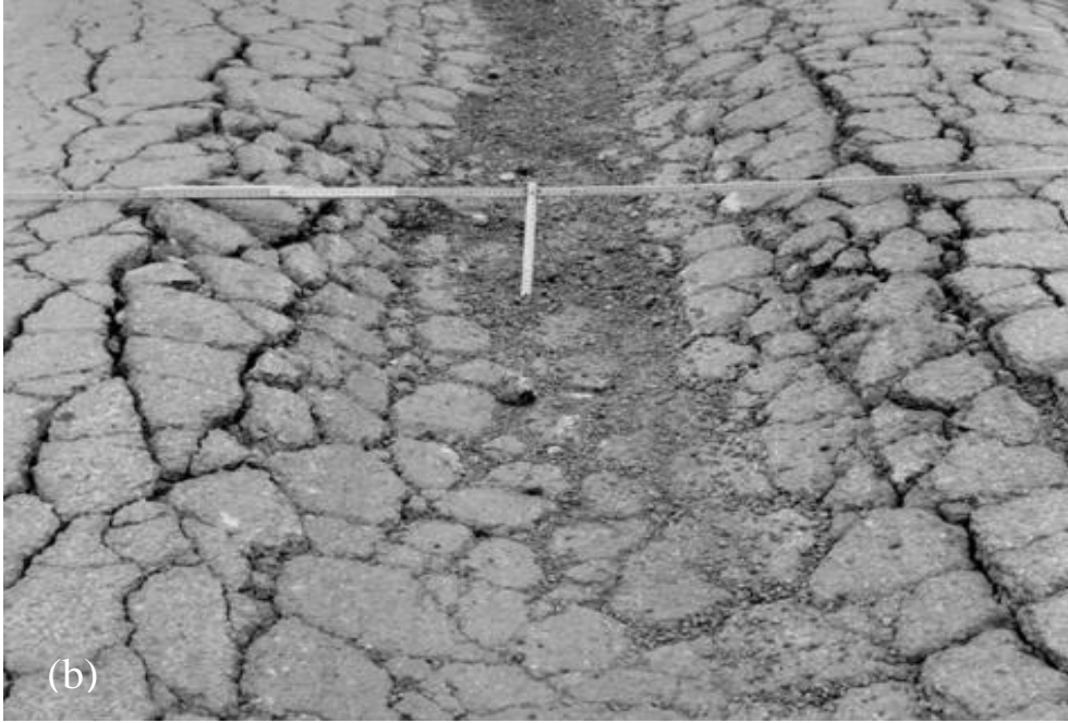
Figure 1-1 Pavement suffering: (a) fatigue cracking; (b) rutting
