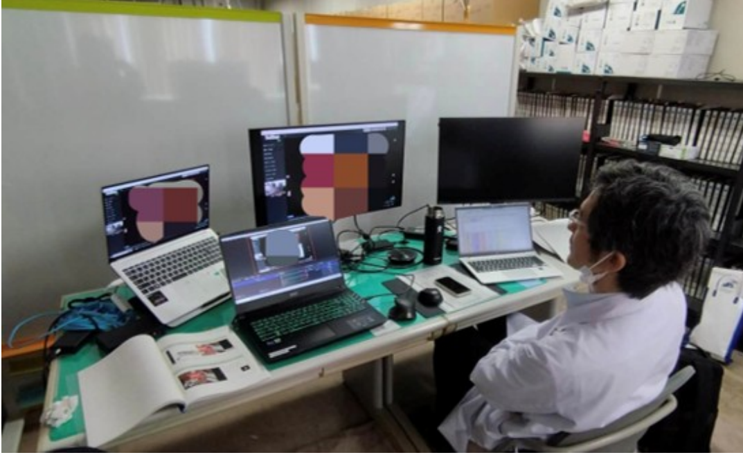
Figure 2.12: Remote mentoring workstation at Hokkaido University (mentor side). The instructor monitors multiple synchronized video streams (endoscopic view, room-side view, and console/robotic view) during the tele-mentoring session with Obihiro Kosei Hospital.
