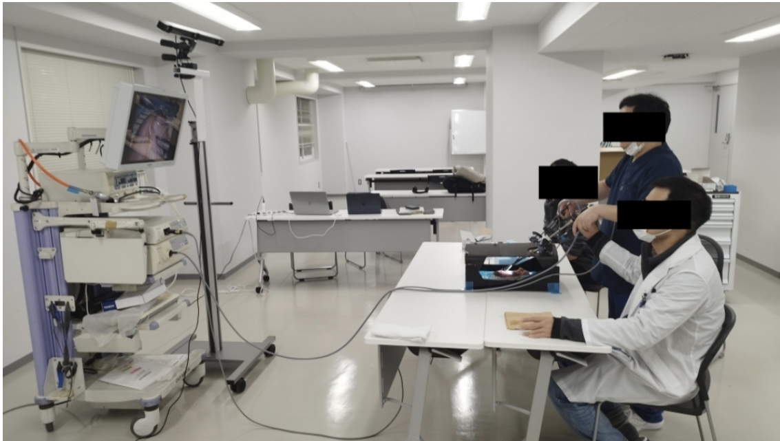
Figure 2.7: Wet-lab experimental setup used at the Simulation Center of Hokkaido University Hospital. Participants performed the tasks in a standing position while using an HD laparoscopic tower and a box trainer equipped with porcine organs. The OptiTrack V120 Trio optical motion capture system was positioned in front of the trainer to record 3D instrument trajectories throughout each task.
