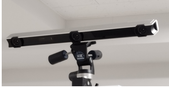
Figure 2.1: Overview of OptiTrack V120:Trio camera system [39]. The device integrates three infrared cameras into a rigid housing, enabling 120 Hz marker-based tracking in a compact surgical workspace.
