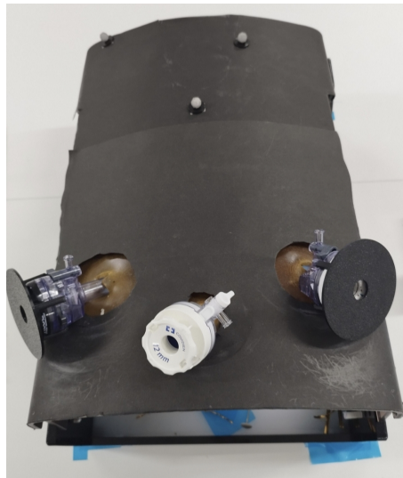
Figure 2.8: Three-port configuration of the box trainer used in the porcine experiments. All ports were 12 mm in diameter, consisting of one central port for the endoscopic camera and two lateral ports positioned at clinically relevant angles for instrument insertion.
