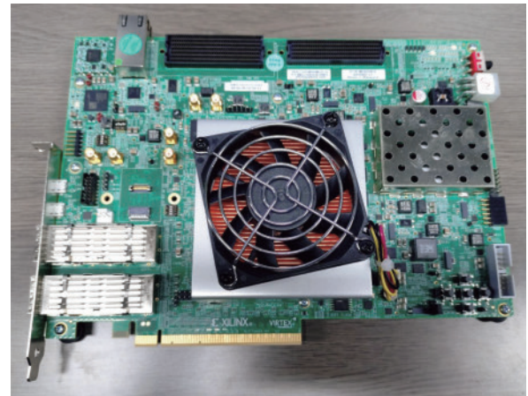
Fig. 3-18. External view of the FPGA.
