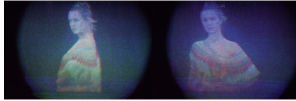
Fig. 3-28. Reconstructed images observed from surrounding viewpoints using real-world captured data.
