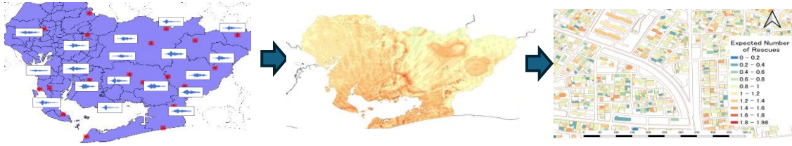
Figure 1 Process for estimating ground motion for each building based on seismometer data
