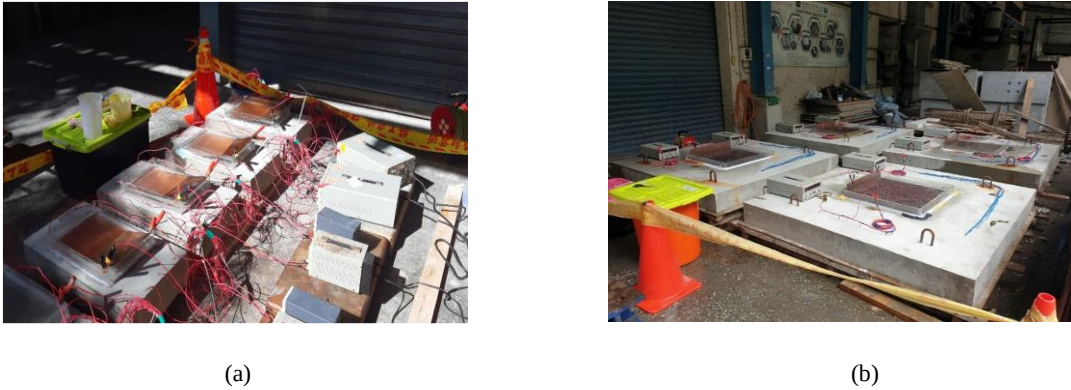
Figure 1. Constant current accelerated corrosion setup; (a) one-way RC slab specimen; (b) two-way RC slab specimens.
