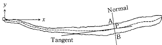
Fig. 9. Calculation method of tuber width using the normal to the center line.
