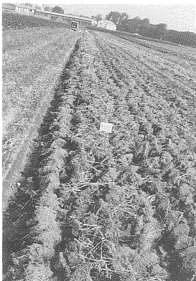
Fig. 10. Soil surface after tilth by type A. ( v=0.4 m/s, PTO 460 rpm, \lambda=7.7 )
