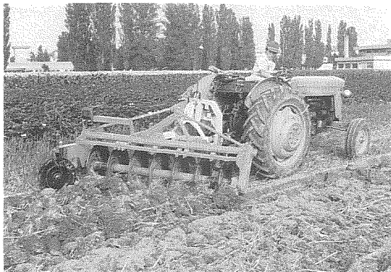
Fig. 8. Field operation of type A (Tractor wheel out of furrow).
