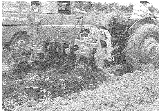
Fig. 9. Field test of type B with additional weight (Tractor wheel in the furrow).
