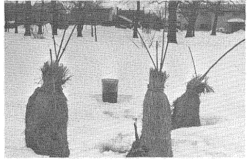
Fig. 2. Plastic bucket for sampling of snowfall with vinyl bag set on the snow surface.
