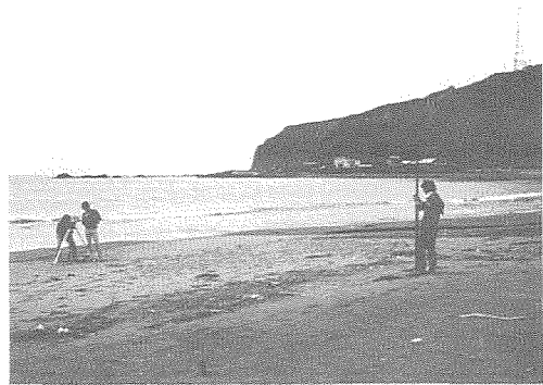
Photo 4. Measurement of the inundation height at Horikappu.
