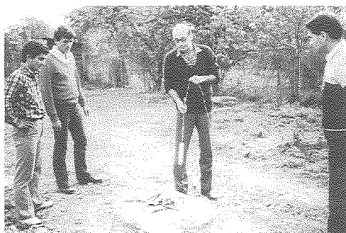
Photo 5. Deployment of the sensor into a Romanian well in October 1985. Simple and low cost twisted wires can be used for the system. The cable has steel conductor wires so that it is strong enough to be used for observations with depth exceeding 1000 m.
