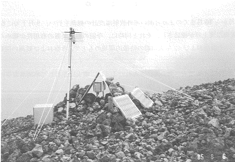
Photo 2. View of telemetering station. Beneath the triangular roof, an infrared radiation thermometer is seen. The background is 62-I Crater.
