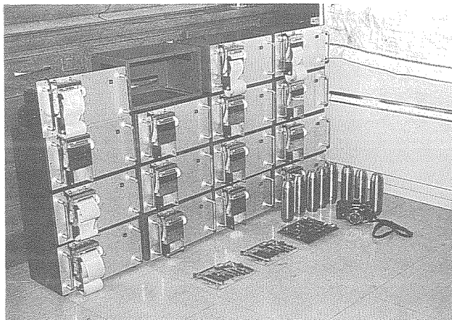
Fig. 1. Developed groundwater thermometers, type 993, which make use of quartz sensor. The sensor is housed in a stainless steel pressure case.
