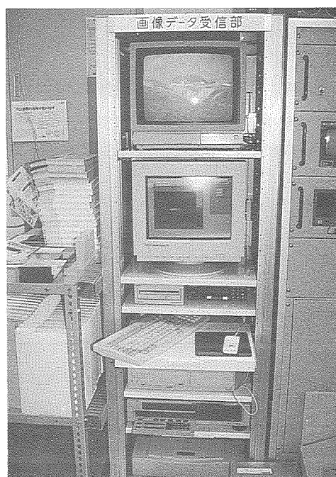
Photo 7 Monitoring system of the infrared and visual images from Mt. Tarumai at UVO.
