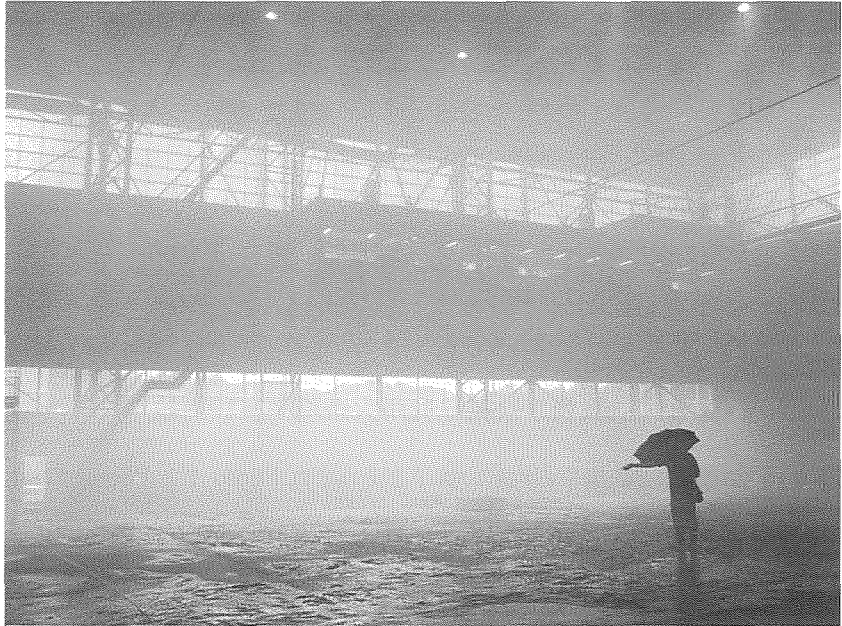
Photo 2. View of an experiment in the NIED rain simulator.
