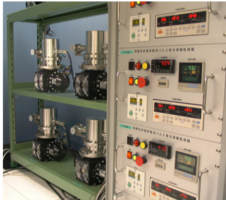
Figure 10. Continuous operation test for evaluating random failure with four identical cryostats.
