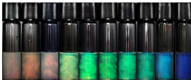
Figure 2. Color change from pink to deep blue with increasing molar ratio of SDS to DGI observed at 3 hrs after mixing SDS and DGI (from left to right, the molar ratios of SDS to DGI are 1:4000, 1:2500, 1:1000, 1:600, 1:400, 1:200, 1:100, 1:75, 1:50, 1:40, respectively)
