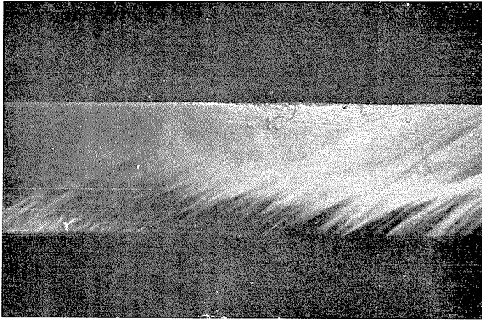
Fig. 7. Single crystal ice having interior distortion. Photograph was taken under the crossed polaroids.
