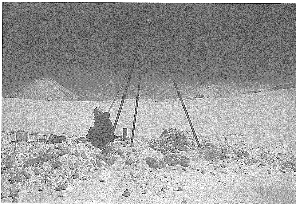
Fig. 7. Drilling site at the center of Gorshkov crater. The tripod was used for supporting the PICO lightweight coring auger. The background is the Kamchatka's highest active volcano, Klyuchevskoy (4750 m a.s.l.).
