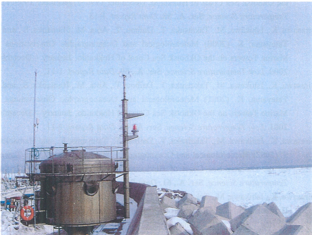
Fig. 2 The Air-Sea-Ice Observation System (ASIOS) tower.
