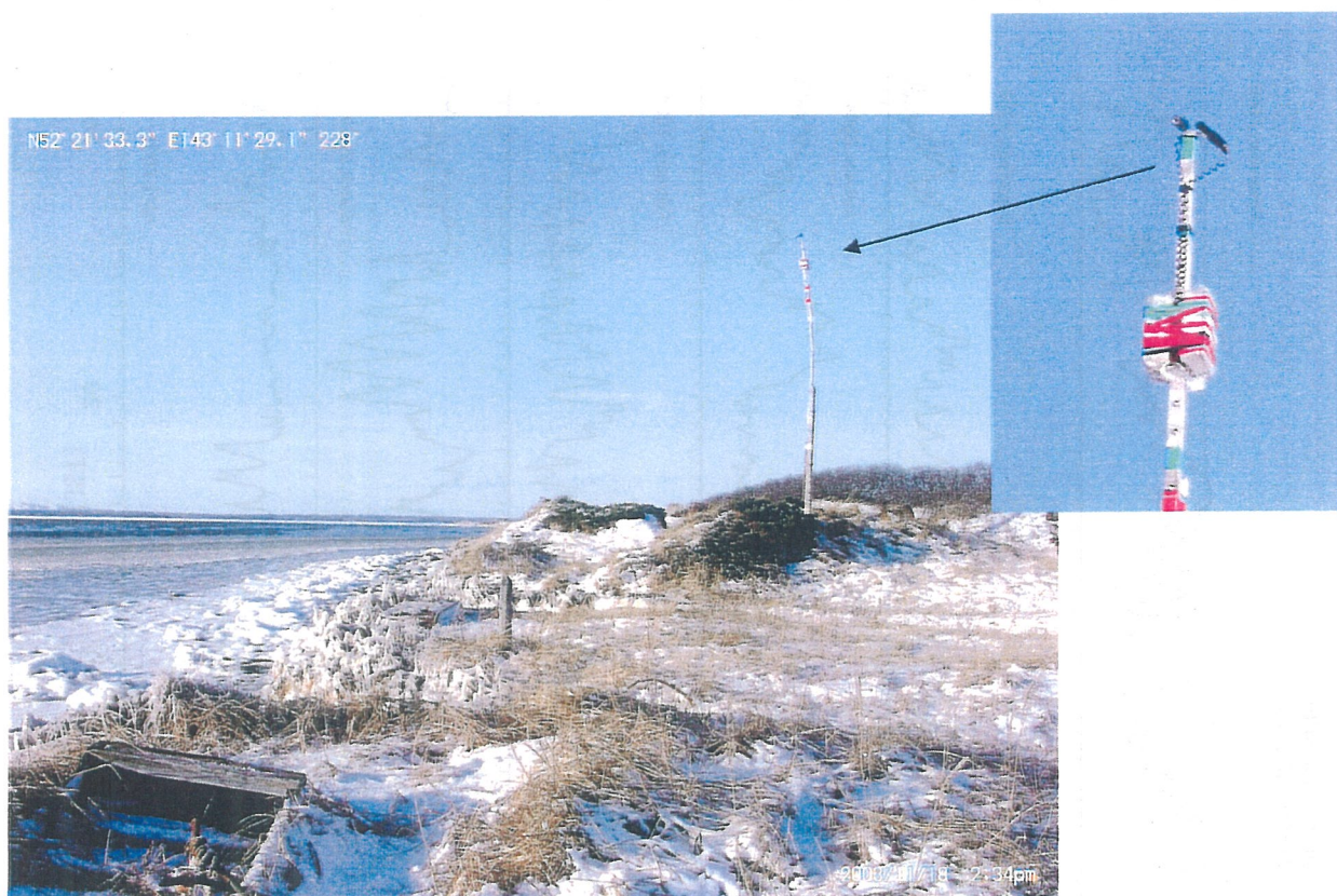
Fig. 2 An automatic weather station (top) and surface radiative temperature sensors installed at the edge of the shore at Kleye Strait near Chaivo Research Station (bottom).
