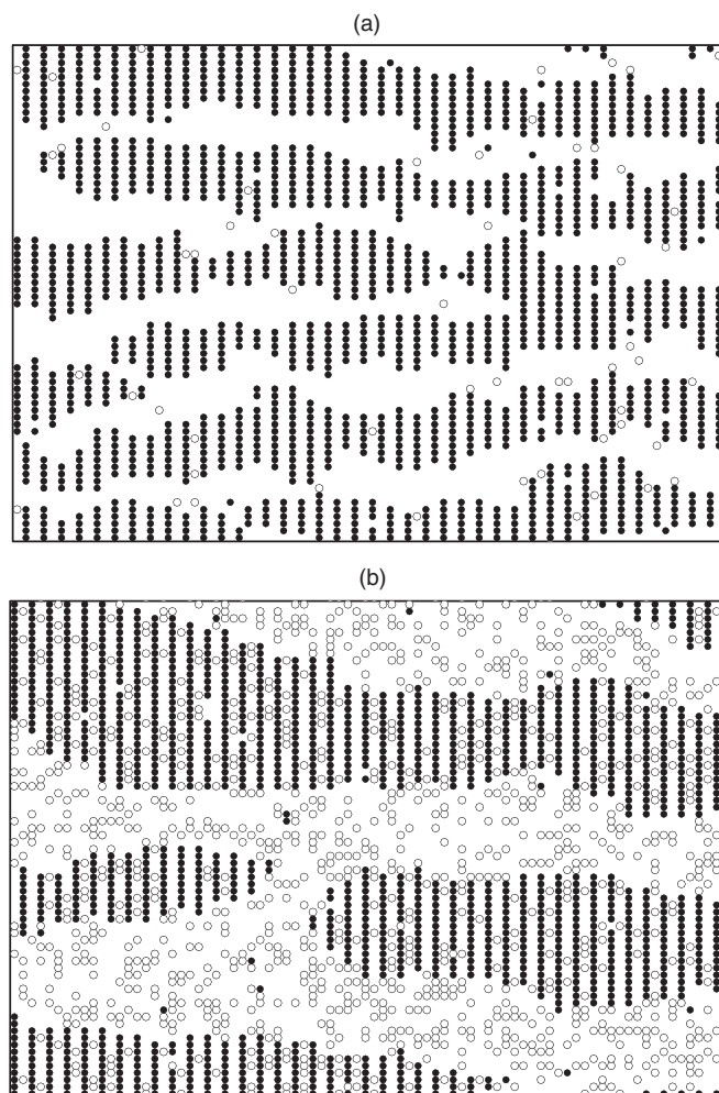
FIG. 3. Snapshots of a 80 \times 70 fragment of the 200 \times 200 lattice during the high reactive regime: (a) at P_{\text{CO}} = 1.8 \times 10^{-7} Torr for the kinetics exhibited in Fig. 1(b); (b) at P_{\text{CO}} = 10^{-7} Torr for the kinetics presented in Fig. 1(c). The solid and open circles indicate O and CO, respectively. The vacant sites are not shown. Note that oxygen atoms form anisotropic (1 \times 2) islands (in reality the formation of such islands is accompanied by rearrangement of surface Pd atoms).
