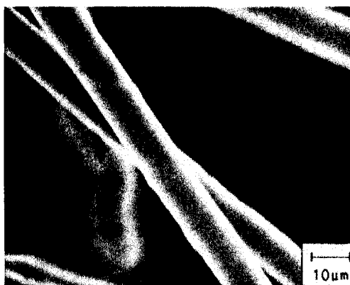
Fig. 5-4 SEM Micrograph of VGCFs (Carbon Source: n -Hexane)
