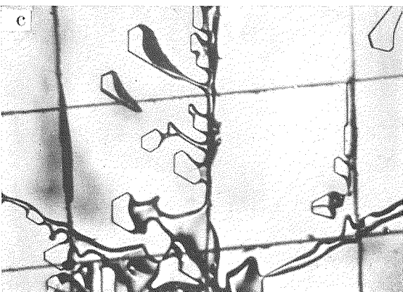
Metamorphosis of snow crystal subjected to a temperature gradient. The arrow shows the direction of heat flow caused by the temperature gradient. Fig. 30 (left) Dendritic snow crystal; -15^{\circ}\text{C} , 0.3^{\circ}\text{C}/\text{cm} ; (a) original crystal, (b) after 24 hours, (c) after 48 hours. Fig. 31 (right) Graupel; -15^{\circ}\text{C} , 0.4^{\circ}\text{C}/\text{cm} ; (a) original graupel, (b) after 34 hours, (c) after 10 days.
