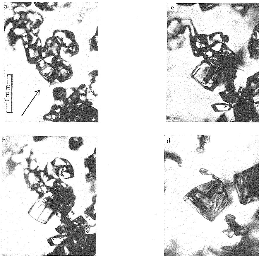
Fig. 33 Development of hoar crystals on the ice grains by an intense temperature gradient 0.7^{\circ}\text{C}/\text{cm} at -15^{\circ}\text{C} . (a) after 3 hours, (b) after 3 days, (c) after 7 days, (d) after 12 days.
