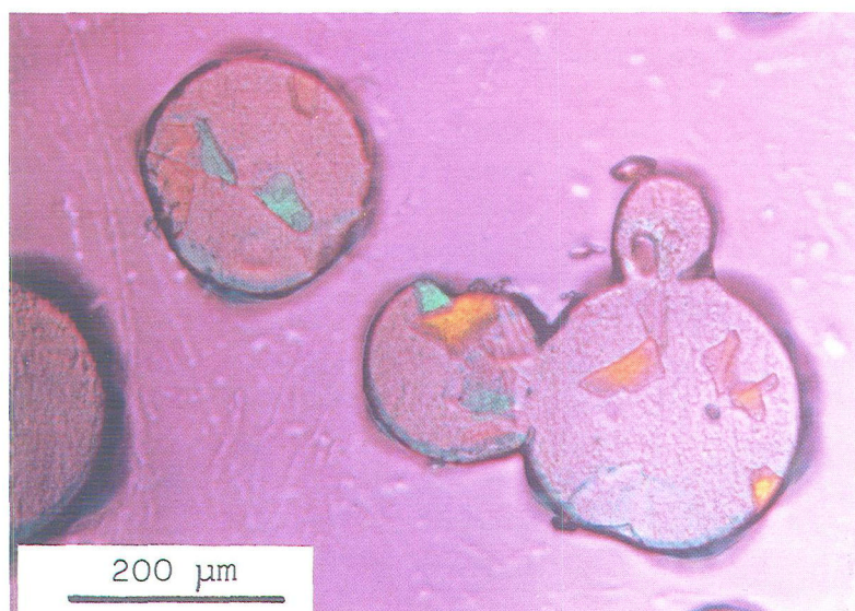
Fig. 2 Microphotograph of polycrystalline droplets frozen on the prismatic plane at -21^\circ\text{C} . Orientation of the largest crystal coincides with that of the substrate.
