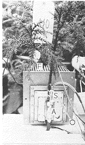
Fig. 1. Thermoelectric apparatus for cooling locally a part on a stem. A, stem part cooled locally (5 cm in length); F, cooling fin of thermoelectric apparatus; O, a lead-wire to a thermocouple; S, needle-type thermister for temperature control
