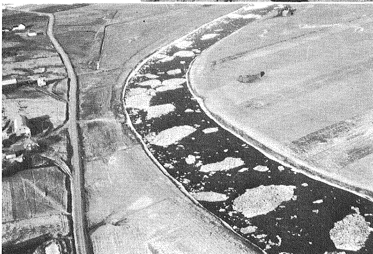
Fig. 5. Successive forms of frazil ice. Chaudière River. December 1963
