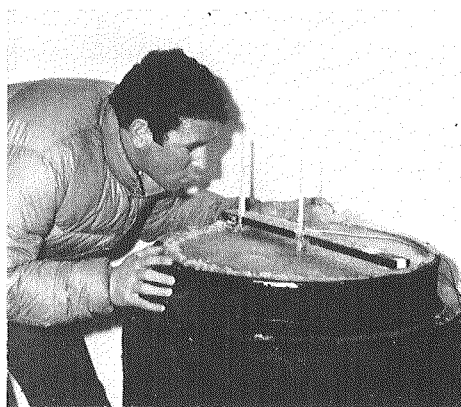
Fig. A 1. Oil drum and frozen sea ice slab in freezer
