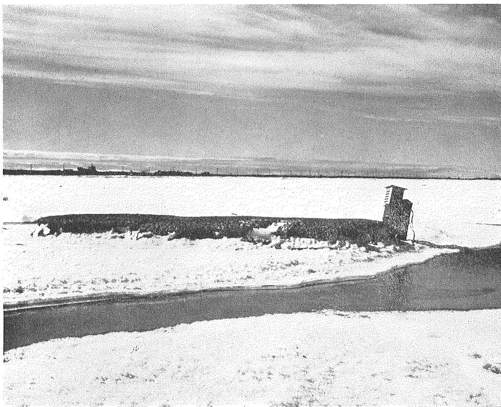
Fig. 3. Ice plot protected by aqueous foam; surrounding ice, which has melted about 1 foot, was originally level with the protected ice surface
