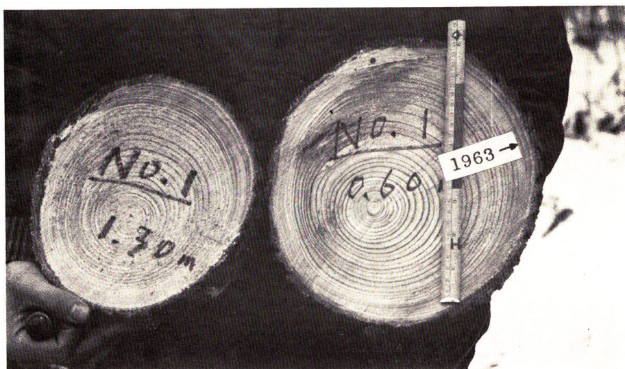
Photo 2. Cross-section of inclined Karamatsu, showing the reaction wood (1963~1964) that formed by sliding in 1962.
