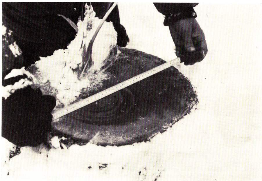
Photo. 17. Cross-section of Akazomatsu ( Picea glehnii ) stem showing scrollshaped reaction wood.
