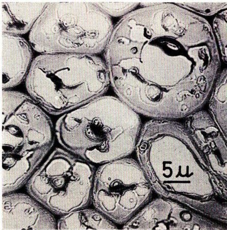
Photo 5. Beech wood fibers of decay by the soft-rot fungus Chaetomium globosum (UV, 280 m \mu ).
