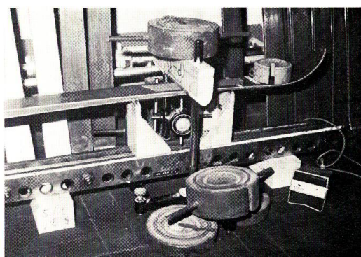
Photo 4. Method of determining the range to be used for bending fracture test within a span.
