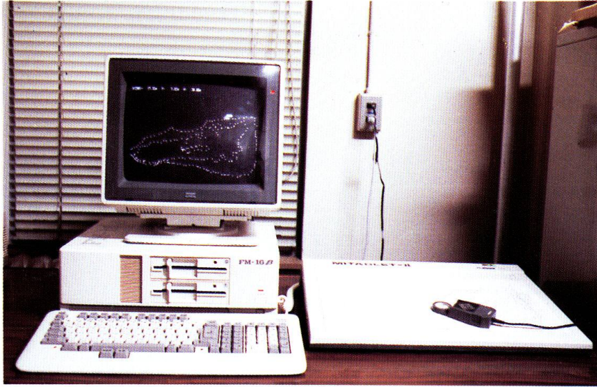
Photo 1. The first stage of input process. (The 3D data of the contour lines traced by the digitizer.)
