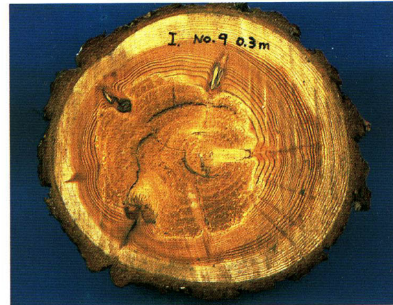
Photo 4. Cross section of a Japanese larch log showing the brown cubical rot caused by Tyromyces balsameus at a height of 0.3 m above the ground.
