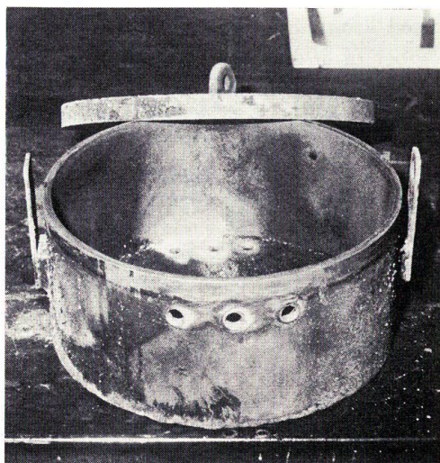
Photo 2. A vessel made of iron for carbonization.
