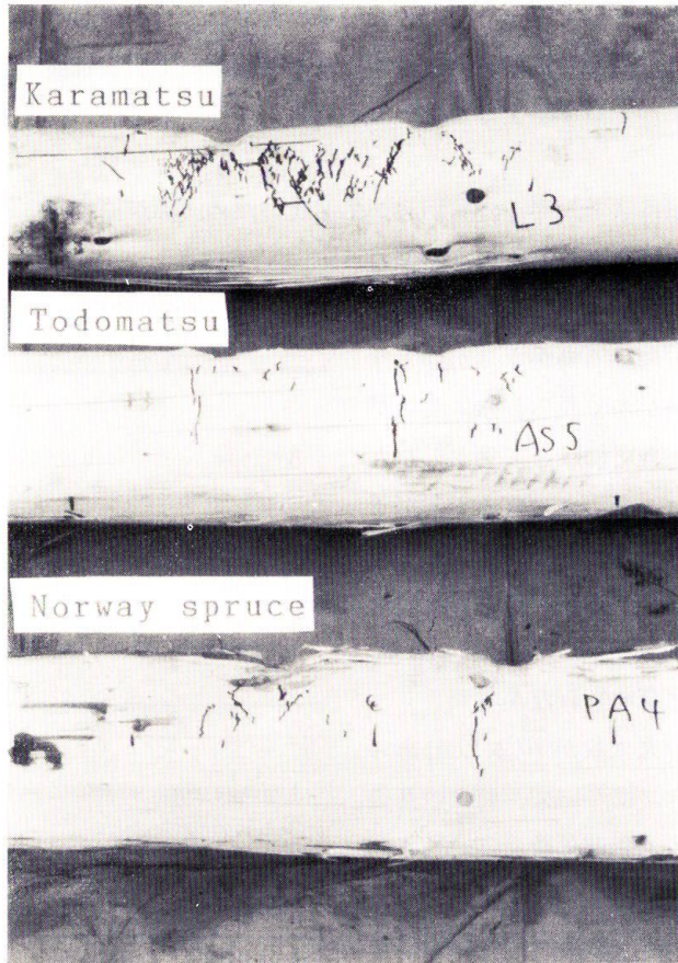
Fig. 11. Typical bending failure of green logs.
