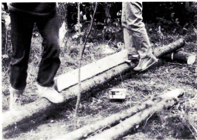
Fig. 1. Bending test in field.
