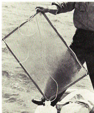
Fig. 31. Stainless steel screen (16-mesh, 50×75 cm.) used for surface skin sampling in Oshoro Bay.
