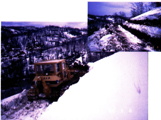
Photo. 4. Making seedbeds on mountainous slopes during snow season. The amount of soil eliminated by bulldozer is small which helps to conserve forest floor.
