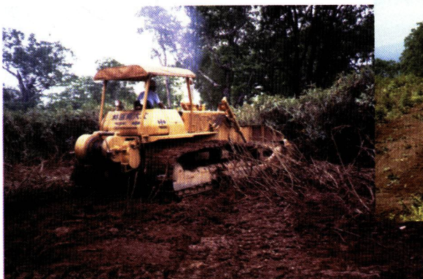
Photo. 7. We employ a bulldozer with upward-warped rakes (a) for site preparation to partly eliminate dwarf bamboo and litter with microorganisms (b).
