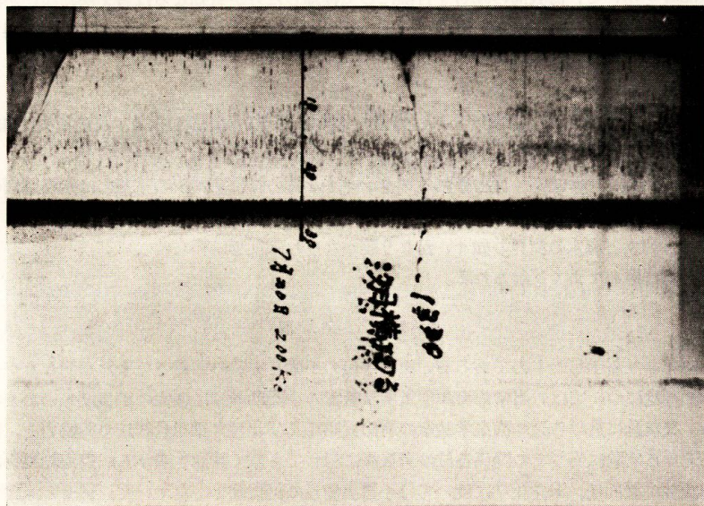
Fig. 18. Sonar echoes due to the bubbles-containing sea water layer under the current rip
