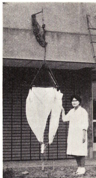
Fig. 3. Original model of triple release mechanism and multiple purse net (Motoda 1962)
