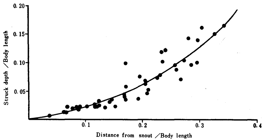
Fig. 12. Relation between the struck depth and the position of the fish (Pink salmon B.L. 45.6 cm) when stuck in the mesh
