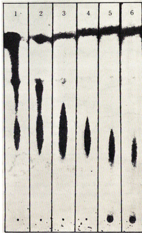
Plate: Kieselgel G, 0.25 mm, activated for 30 min. at 110°C Solvent: n-BuOH-ethyleneglycol-H 2 O (4 : 1 : 2, upper phase) Detection: Hanes-Isherwood reagent Fig. 2 Thin layer chromatogram of each eluted fraction
