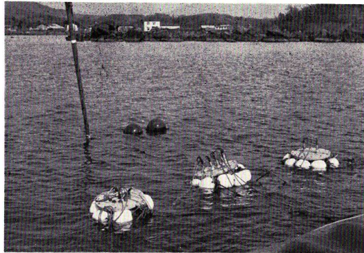
Fig. 6. Mooring buoy of telemeter and device for measuring acceleration.
