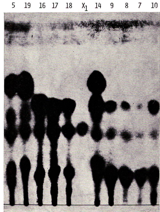
Fig. 4. Paper chromatogram of red algae. Conditions are same as Fig. 3 Detected under light source 3 Numerals refer to Table 1
