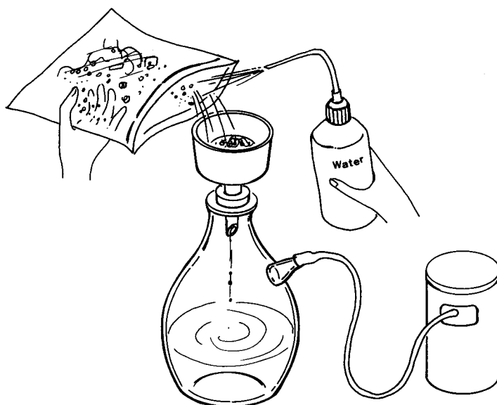
Fig. 2. Transferring a plastic debris sample to a filter paper set in a Buchner type funnel.
