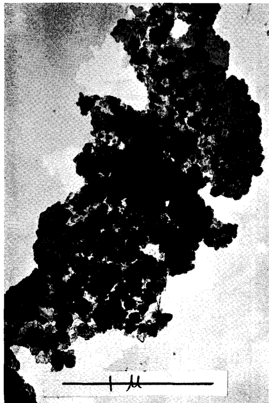
Fig. 12 Replica of basic \text{ZnCrO}_4 at about 600^\circ\text{C} .
