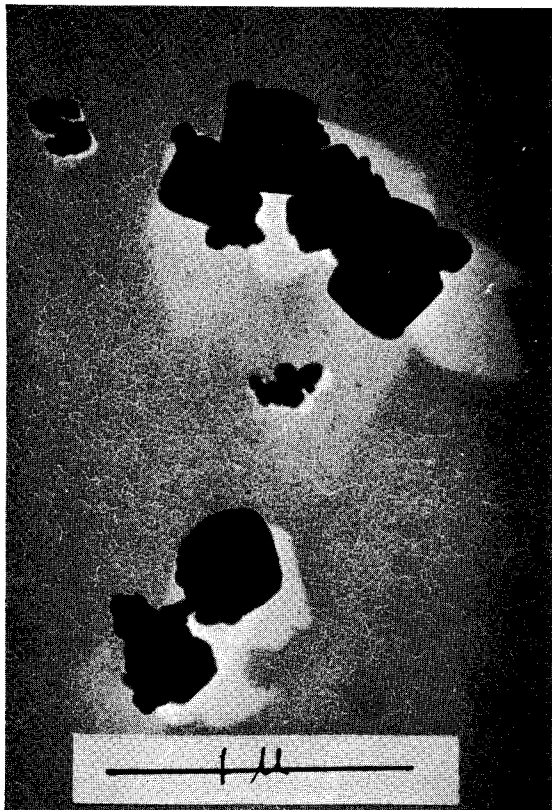
Fig. 20 The polygonal ZnCr_2O_4 particles on a collodion film (Cr-shadowing).
