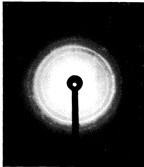
Fig. 10 The selected-area electron diffraction pattern of the colloidal particles (see the arrow in Fig. 9).
