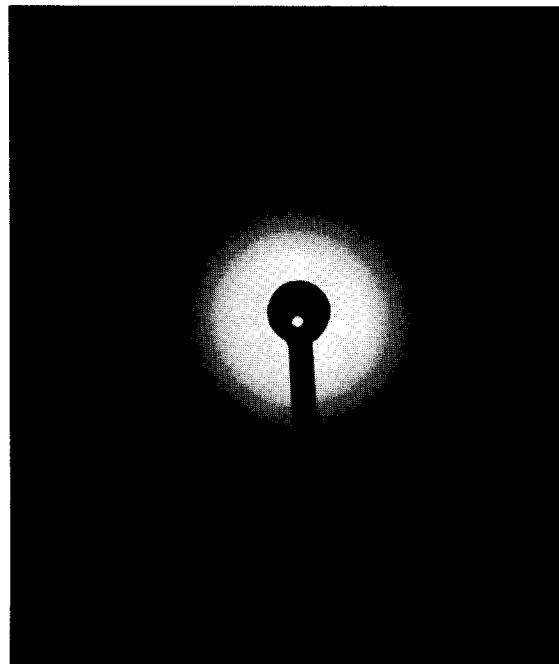
Fig. 19 The selected-area electron diffraction pattern of the transparent area in Fig. 17a. This pattern is ascribable to the amorphous carbon film (see the arrow in Fig. 17a).
