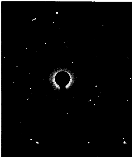
Fig. 18 The selected-area electron diffraction pattern of the opaque colloidal particles in Fig. 17b. This indicates a small amount of randomly disposed ZnCr 2 O 4 crystallites (see the arrow in Fig. 17b).
