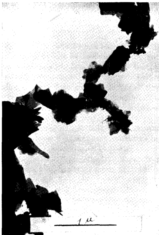
Fig. 1 a Basic \text{ZnCrO}_4 on a collodion film.
