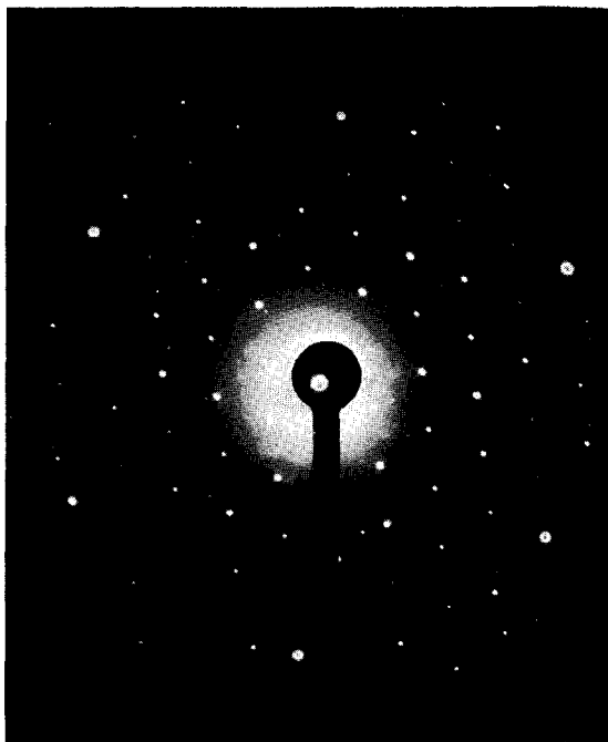
Fig. 1 b Selected-area electron diffraction pattern of a single crystal of basic ZnCrO 4 . S_0 // (001)-axis of basic ZnCrO 4 .
