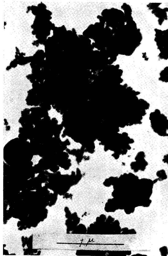
Fig. 14 The "reduced" catalyst on a collodion film. Note fringes surrounding the particles.
