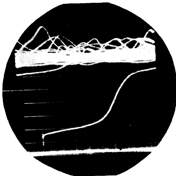
Plate 2. The potential-time variation after switching on a polarizing current on an evaporated platinum film electrode in aqueous \text{Na}_2\text{SO}_4 , pH 2.83; the ordinate 100 mv/Div, the abscissa 5 m sec/Div, i = 8.7 \cdot 10^{-2} amp \cdot\text{cm}^{-2} .
