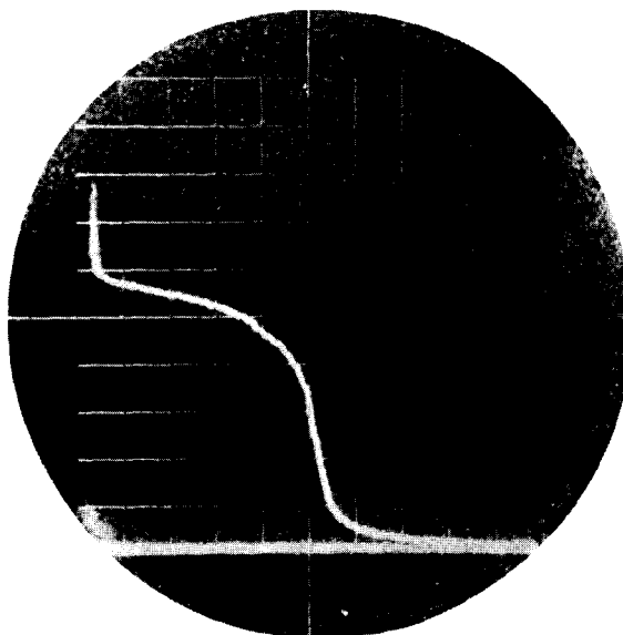
Plate 3. The potential-time variation after switching off a polarizing current on an evaporated platinum film electrode in aqueous \text{Na}_2\text{SO}_4 , pH 2.83; i = 1.35 \cdot 10^{-1} amp \cdot\text{cm}^{-1} , the ordinate 100 mv/Div, the abscissa 100 msec/Div.
